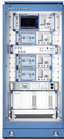
The R&S®TS6710 test system for development and production measures the main parameters of transmit/receive (T/R) radar modules in less than 15 seconds (2500 test values) and performs a complete characterization (> 25000 test values) in less than 4 minutes.
