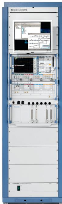
Modular, complex microwave switching matrices, including software for calibration and automatic single-ended integrity check
