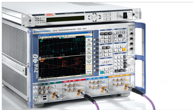
Digital frontend of the R&S®ZVA to measure the phase difference of signals with different frequencies
