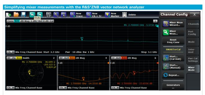
The four-port R&S\*ZNB vector network analyzer fitted with a second internal generator, together with the mixer measurement wizard and SMARTerCal, measures important mixer parameters up to ten times faster and more accurately, such parameters including conversion loss (top) as well as RF input (S11) and IF output (S22) return loss (bottom left and right respectively).
