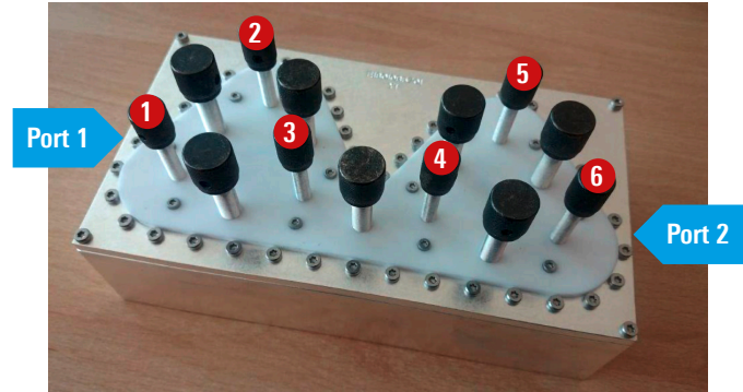
Fig. 3: Filter with numbered resonators.
