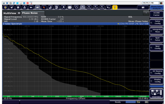
The R&S®FSWP displays the achievable level of sensitivity with gray color-coding.
