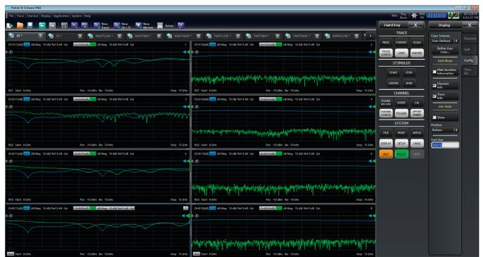
All ports of the beamforming IC at a glance using the R&S®ZNBT multiport VNA
