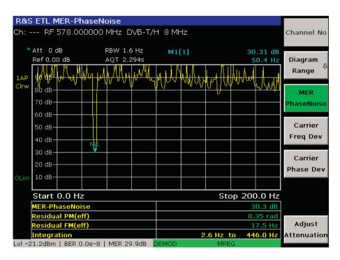
The new and unique MER phase noise measurement capability of the R&S°ETL shows the causes of the poor MER of 29.9 dB at a glance (center of the bottom status bar): In this case, the unwanted phase noise at 50 Hz (see M1) primarily determines the signal quality.
