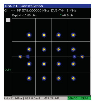
This figure shows the proven MER measurement for a DVB-T signal that was mainly affected by unwanted modulator phase noise. The cause cannot be seen in the constellation diagram. The R&S<sup>®</sup>ETL can make the cause visible with a new unique measurement capability.
