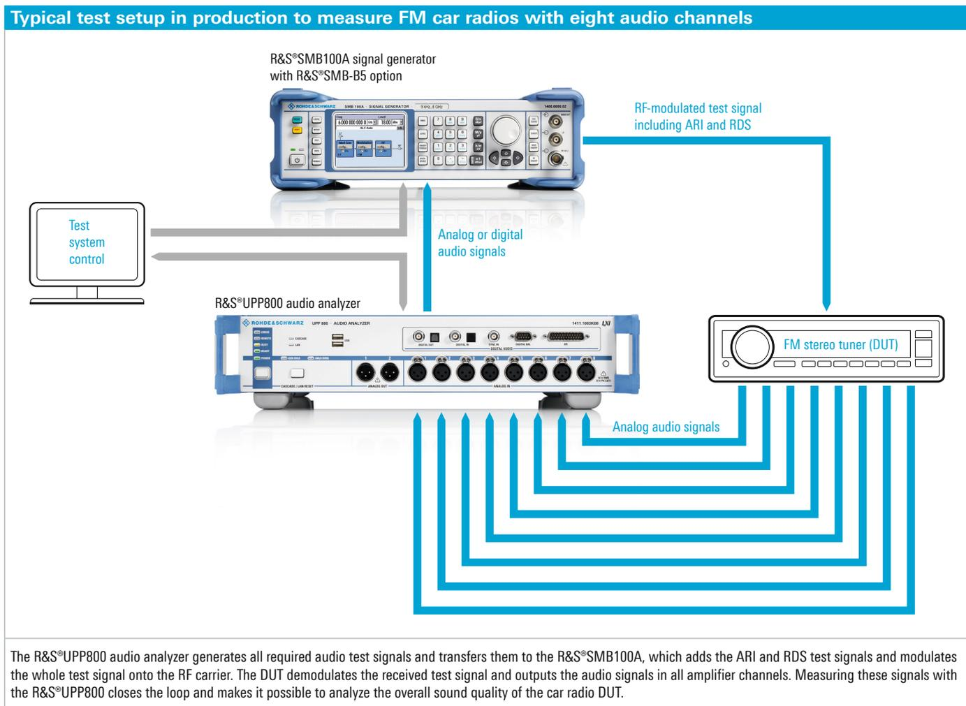
The R&S®UPP800 audio analyzer generates all required audio test signals and transfers them to the R&S®SMB100A, which adds the ARI and RDS test signals and modulates the whole test signal onto the RF carrier. The DUT demodulates the received test signal and outputs the audio signals in all amplifier channels. Measuring these signals with the R&S®UPP800 closes the loop and makes it possible to analyze the overall sound quality of the car radio DUT.
