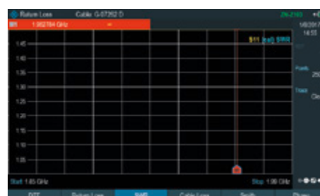
Fig. 5: VSWR measured with open circuit, VSWR = ∞.
