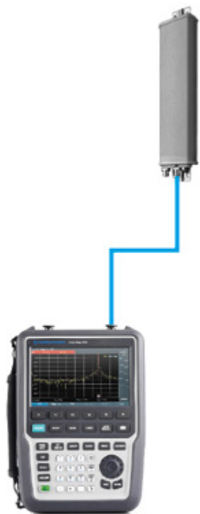
Fig. 1: Reflection measurement of a base station antenna with R&S®CableRider ZPH.
