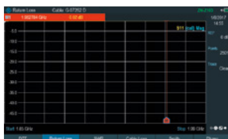
Fig. 4: Return loss measured with open circuit, return loss = 0 dB.
