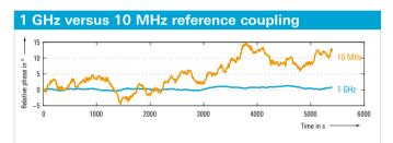
The phase stability of 1 GHz reference coupling (blue) is significantly better than 10 MHz coupling (orange) at 6 GHz RF output and constant temperature over 90 minutes.
