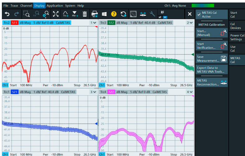
S-parameters for a 40 dB attenuator with measurement uncertainty bands.
