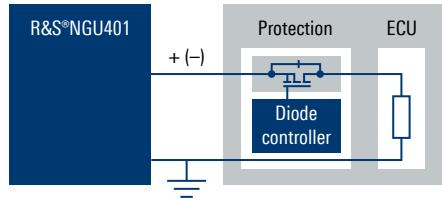
Using a diode controller with an N-channel MOSFET will produce the lowest reverse current. However, this solution requires the ability to measure current of less than a few nA in the reverse mode.
