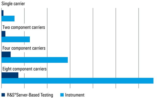
In both cases, the instrument executed both the auto amplitude leveling and the I/Q capturing. The signal analysis time increases proportionally to the number of component carriers. Each carrier analysis is independent and can be analyzed in parallel with other carriers on R&S®Server-Based Testing. The figure above shows that test times for measurements with eight component carriers are reduced by 89% when using R&S®Server-Based Testing compared to the instrument only scenario.
