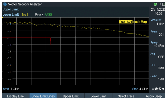
Fig. 2: S_{21} insertion loss measurement.
