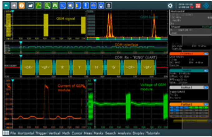
Timing analysis of data capture, processing and communication of a wireless module.
