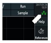
I Touch the green LAN icon on the oscilloscope's display and select parameters to find the IP address. If you need a fixed IP address, change the IPI mode to manual and enter the specified IP address
