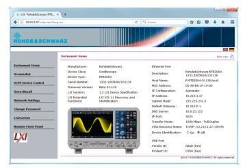
Click "Livescreen" in the menu on the left to obtain a continuously updated image of the oscilloscope display in your browser (the browser can be resized). You can use the "Remote Front Panel" to fully operate the instrument
