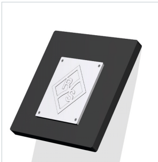
Example radome. The Rohde & Schwarz logo is 600 µm thicker than the base plate to cause RF mismatch at 77 GHz.
