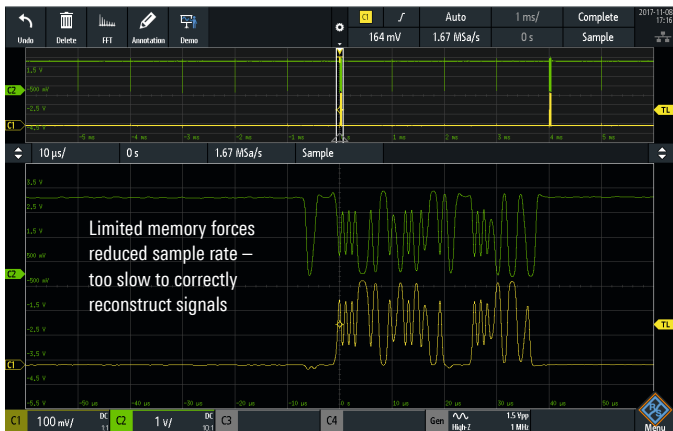
With insufficient memory, the oscilloscope begins reducing sample rate in order to capture more time. This can lead to insufficient sample rates to accurately show signals.
