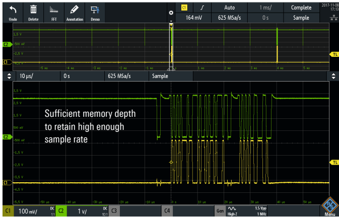
With sufficient memory, the oscilloscope can retain full sample rate (and rated bandwidth) to accurately show the signal.
