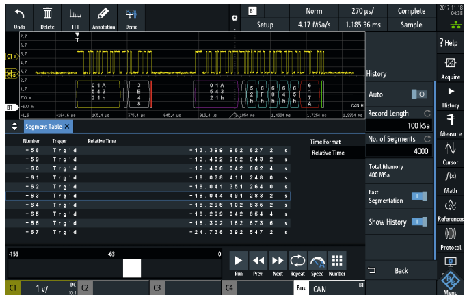
Using segmented memory, the R&S®RTA4004 captures several CAN bus bursts over 87 s.
