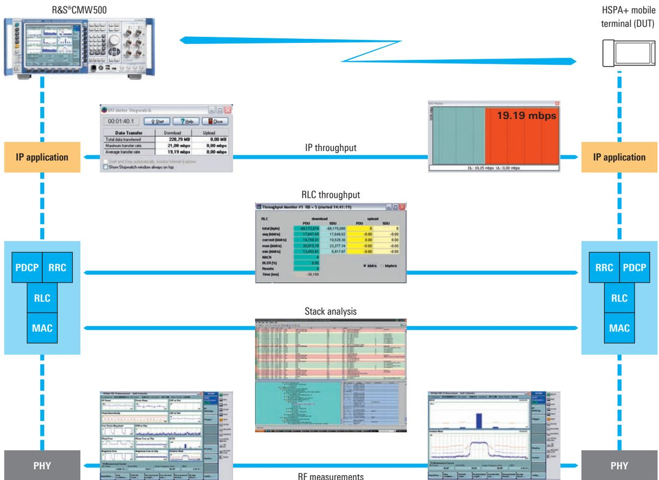
Parallel measurement of all relevant parameters with the R&S®CMW500: The throughput monitor provides performance on the RLC layer while, additionally, bitmeter applications provide E2E performance on the IP layer. Parallel uplink RF measurements can be started in addition.
