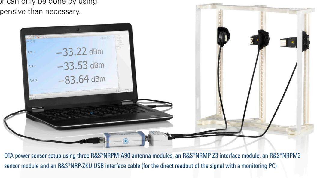
OTA power sensor setup using three R&S®NRPM-A90 antenna modules, an R&S®NRMP-Z3 interface module, an R&S®NRPM3 sensor module and an R&S®NRP-ZKU USB interface cable (for the direct readout of the signal with a monitoring PC)
