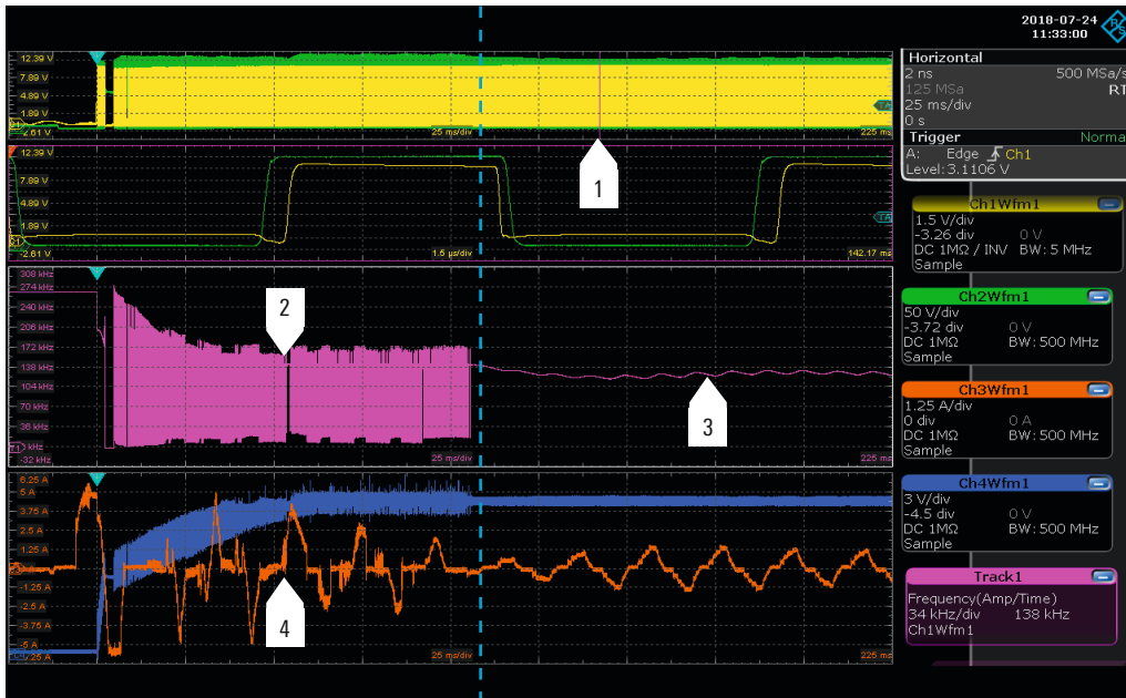
Startup behavior of an LLC resonant converter:
