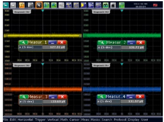
Graphic 4: Low inherent noise, even at a vertical input sensitivity of 1 mV/div.
