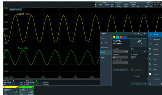
Automatic detection of the R&S®RT-ZPR20 power rail probe on the R&S®RTO6 oscilloscope.
