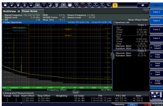
PSNR measurement of a 156.25 MHz oscillator: example, starting with an injection frequency of 3 kHz.
