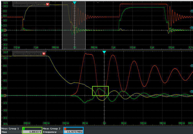
Measurement result of a half bridge configuration
