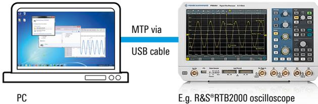
Connect the USB type B device port on the rear of the oscilloscope to a PC USB host port and use the following features:
