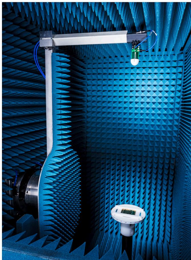
The R&S®ATS1000 includes a high-precision positioner in order to get the 3D data
