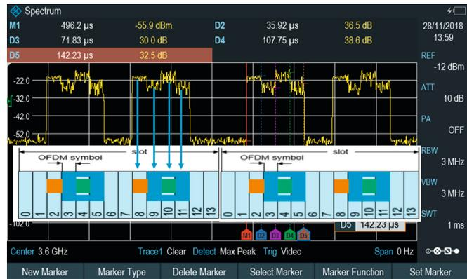
Figure 3: 5G downlink signal with user data in time domain, SC spacing
