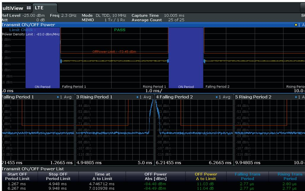
The R&S®FSW with the R&S®FSW-K104 measurement option offers maximum timing accuracy to make ON/OFF power transients of TD-LTE base stations visible.
