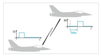
Communications links over long distances cause signal delays that challenge military waveform and radio designs.
