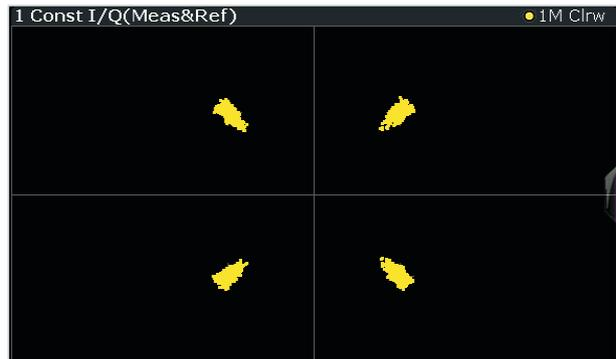
The same signal with strong distortion. It has poor modulation quality, but it is clear that no symbols would fall in an adjacent quadrant.
