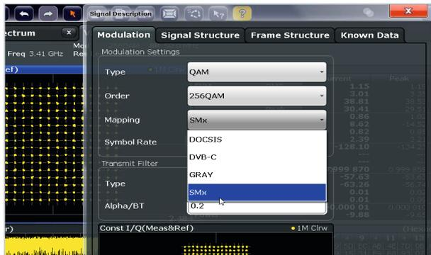
Next, we need to tell the R&S®FSW that it will use "Known Data" for its demodulation process and select the data source and type.
