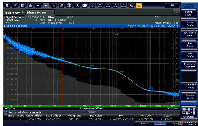
PCIe clock without SSC: phase noise and weighted jitter.
