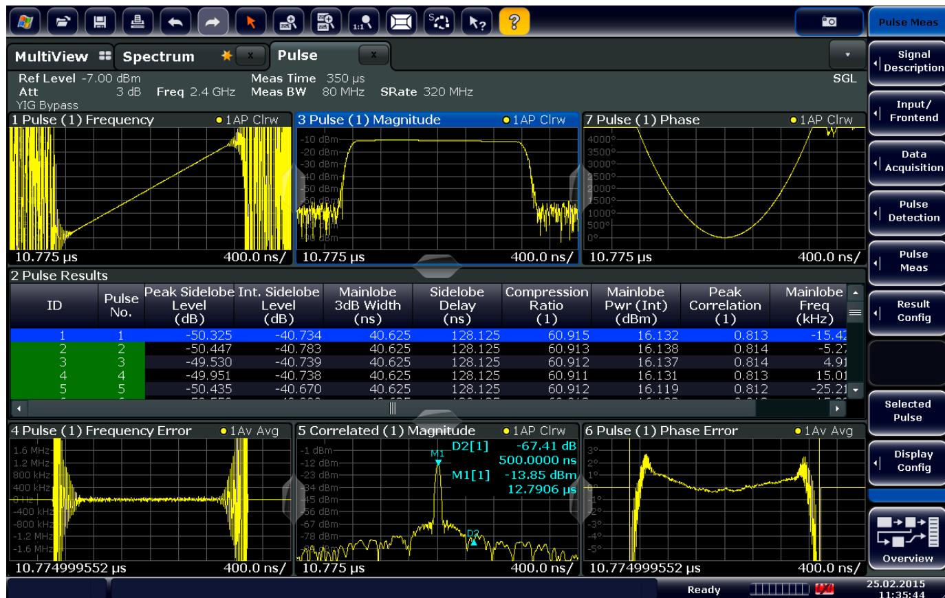
The R&S®FSW displays the correlated magnitude, frequency and phase error traces as well as pulse compression parameters for a linear frequency modulated waveform.
