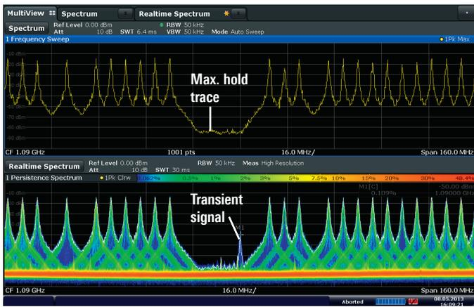
Comparison of a fast hopping radio signal displayed on the R&S®FSW in conventional spectrum analyzer mode (upper) with max. hold trace after several seconds and in realtime mode (lower).
