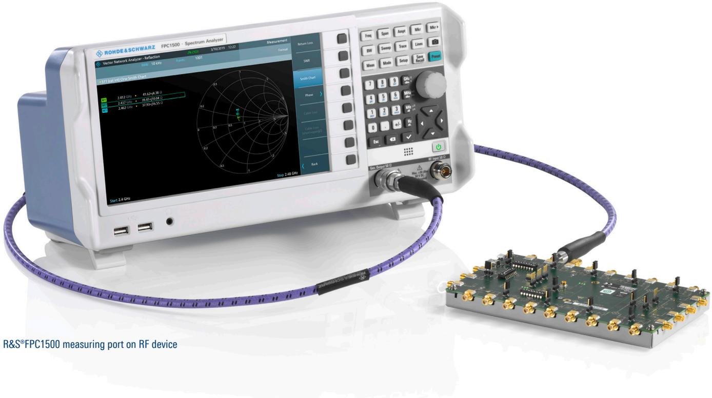
R&S®FPC1500 measuring port on RF device
