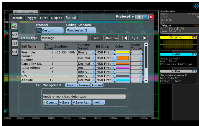
Fig. 3: Format details of the extended squitter message.
