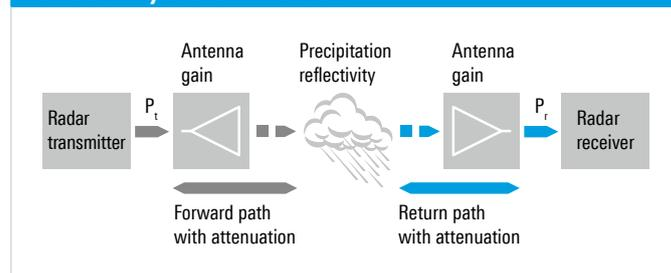
Radar transmitters usually generate sufficiently accurate output power to determine reflectivity. With receivers, this is more difficult. In general, they are able to monitor level changes with high accuracy, but they are characteristically too inaccurate for measuring absolute levels.
