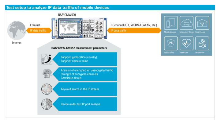
The R&S°CMW500 wideband mobile communication tester with the R&S°CMW-KM052 IP connection security analysis option enables users to identify vulnerabilities in an loT device's IP connection security at an early stage of development.
