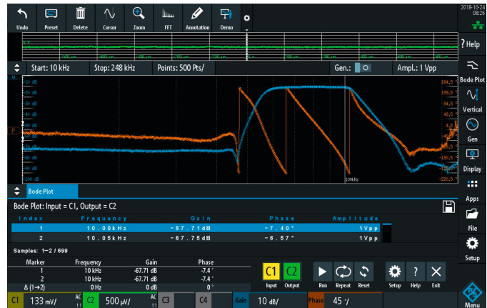
Frequency response of a bandpass filter (blue trace: gain; orange trace: phase)
