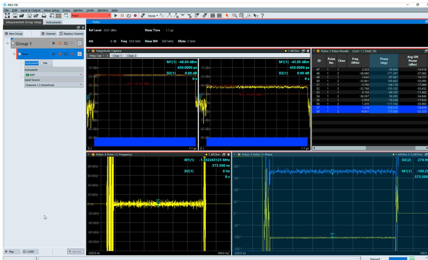
Fig. 4: Main analysis view of the R&S®VSE-K6A multichannel pulse analysis option. The phase difference can be determined either via markers (bottom right window) or from the values in the results table (top right window).
