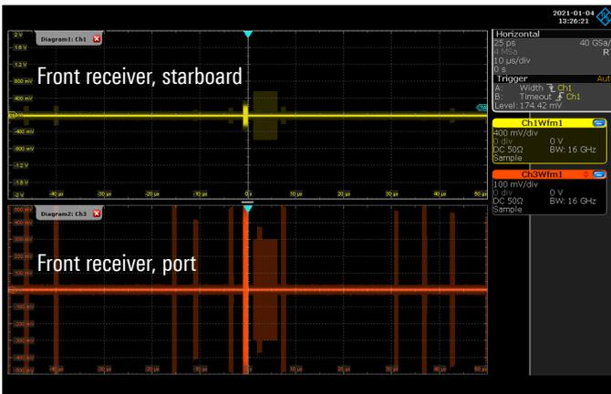
Fig. 3: With only auto trigger in place, a stable trigger condition is not achieved. However, a first overview of the scenario can be established to find proper trigger conditions.
