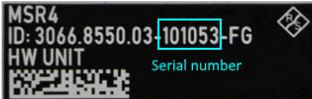
Figure 10: MSR4 unique device identifier on the rear panel
