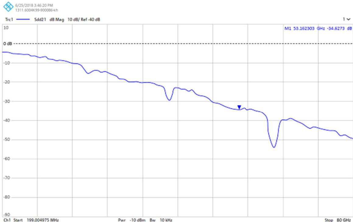
Figure 3:  $|S_{dd21}|$  vs frequency, the insertion loss response of a typical differential high-speed serial circuit.
