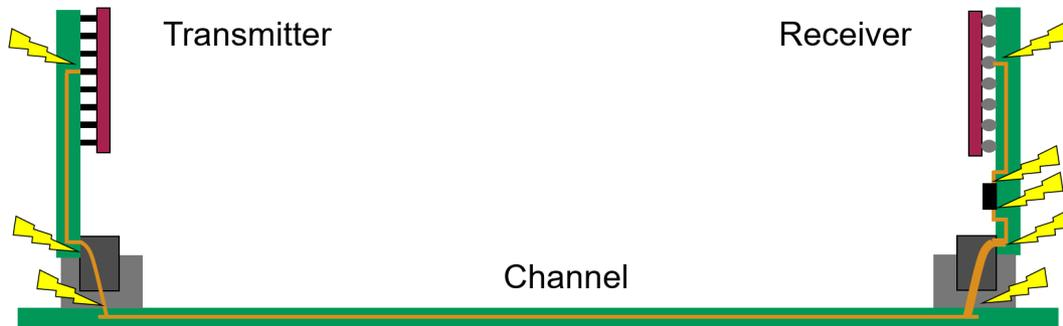
Figure 15: Long reach configuration with multiple discontinuities and corresponding reflections.
