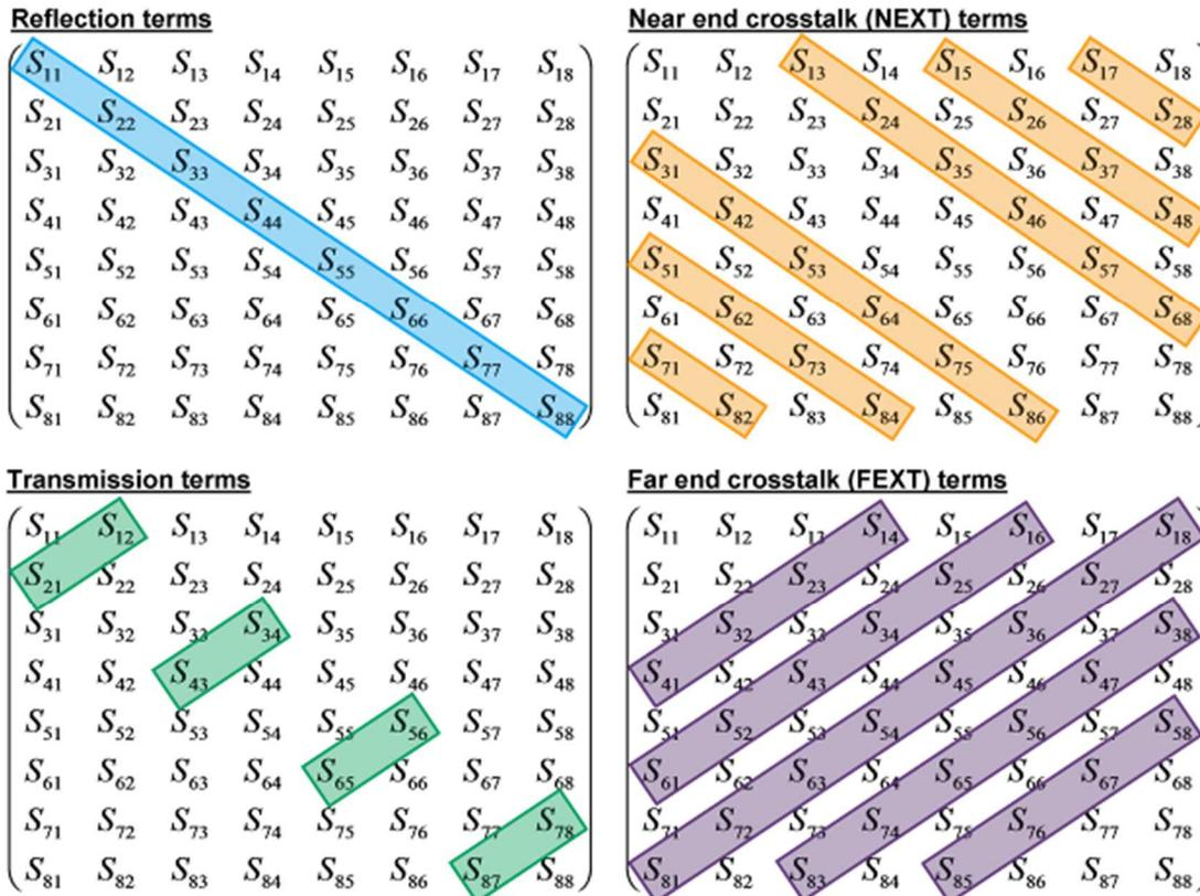
Figure 7: The matrix of S-parameters for a 4 lane system with transmission, reflection, NEXT and FEXT terms indicated.
