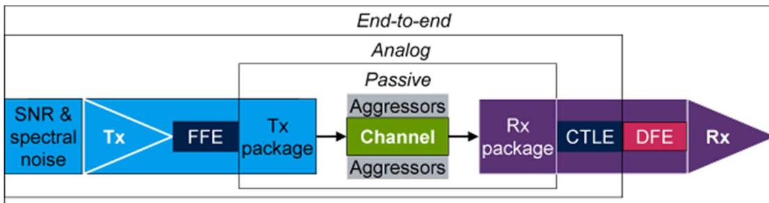
Figure 17: Separating the elements of an IBIS-AMI simulation.
