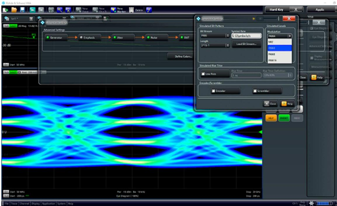
Figure 12: PAM-4 eye diagram calculation.
