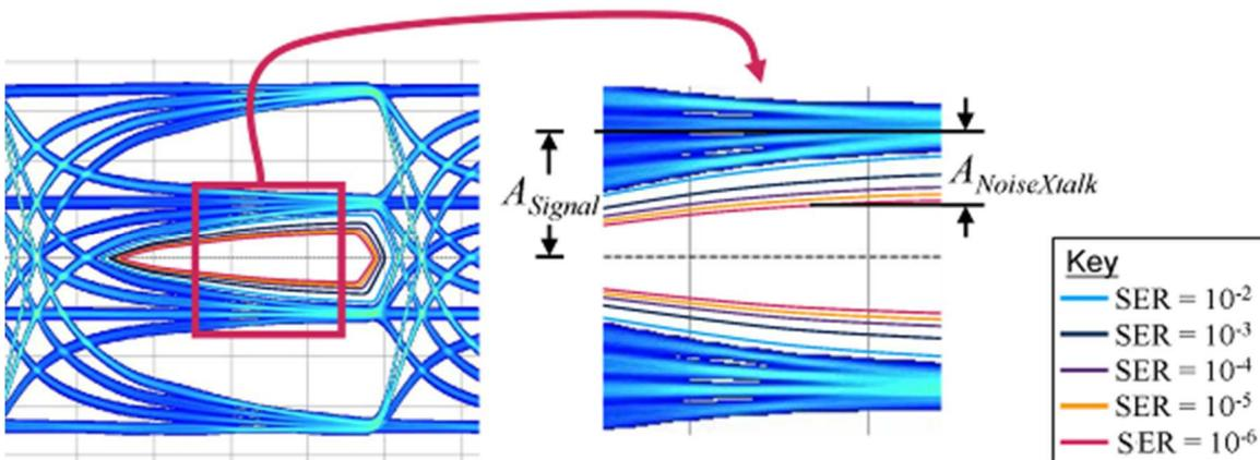
Figure 14: COM is an SNR-like parameter calculated from an eye diagram derived from the pulse response of a system model that is defined by the channel S-parameters.
