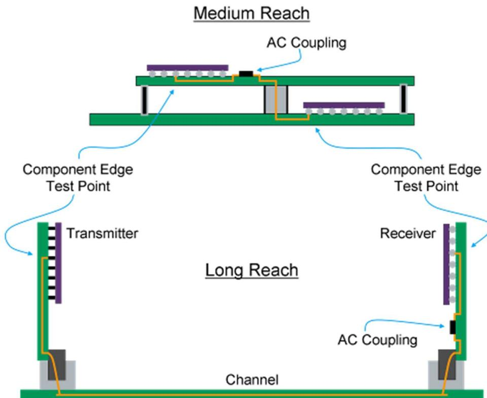
Figure 8: Medium and long reach configurations.
