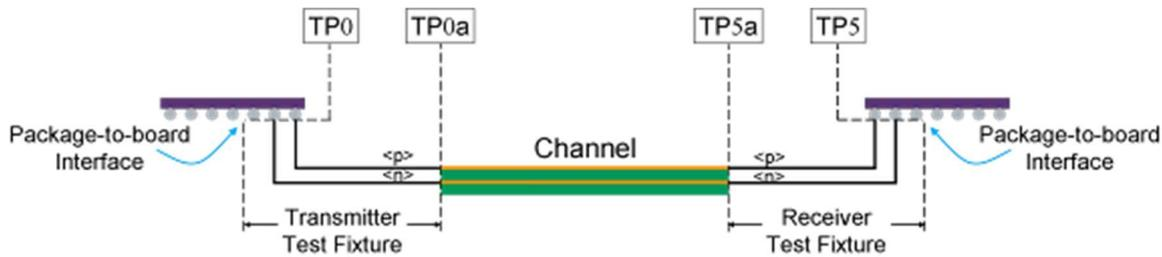
Figure 9: The channel model and test points.
