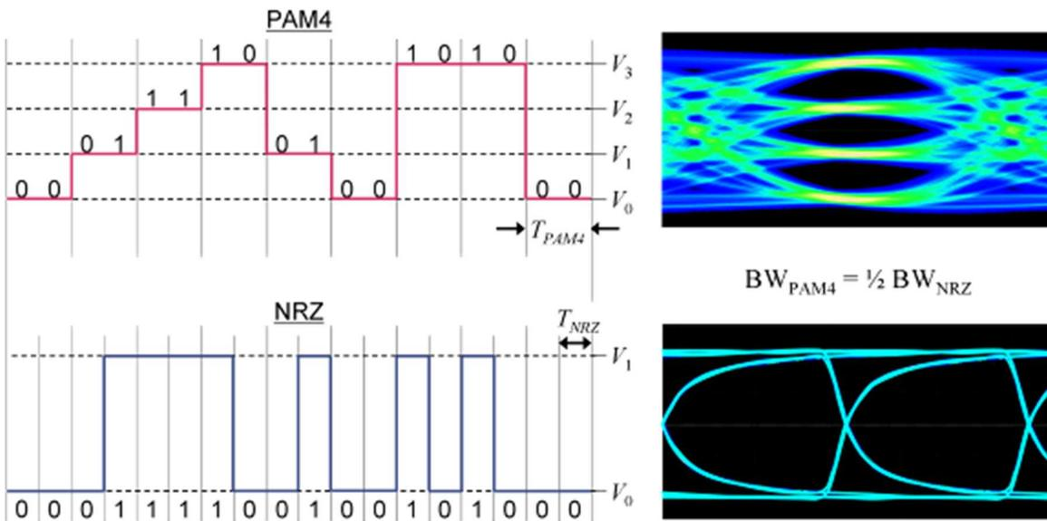
Figure 1: (a) A PAM-4 signal and (b) the equivalent NRZ signal.
