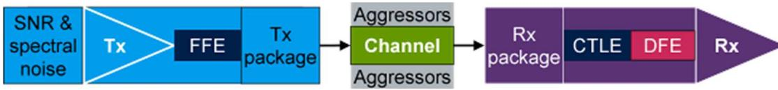
Figure 13: Elements of the COM calculation.
