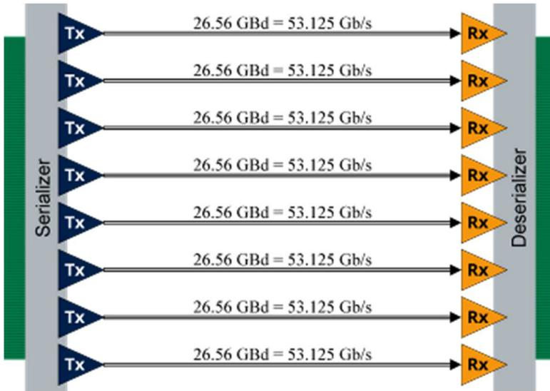
Figure 2: Example of a 400 Gb/s system, 400GAUI-8.
