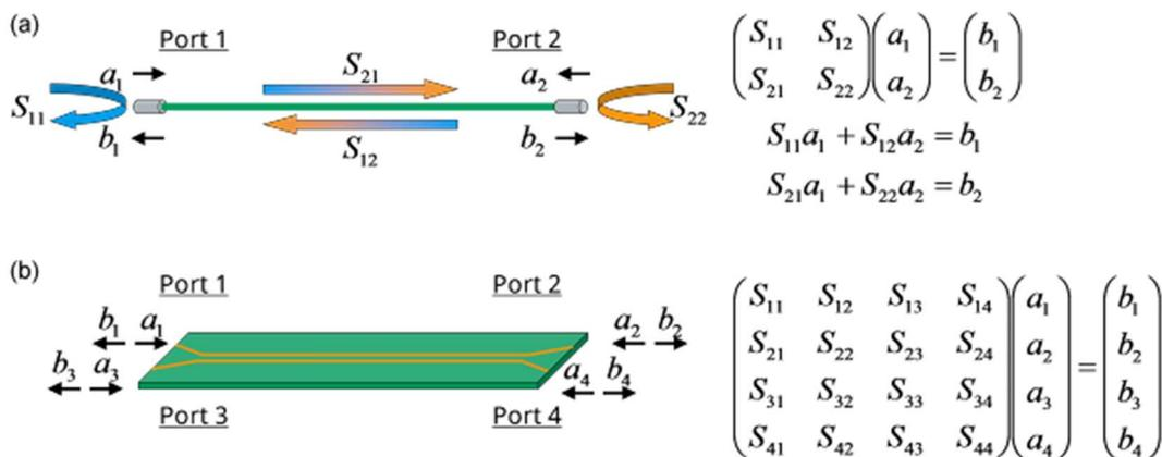
Figure 5: S-parameters: (a) 2x2 S-parameter matrix for a single trace or cable and (b) 4x4 S-parameter matrix for two channels.
