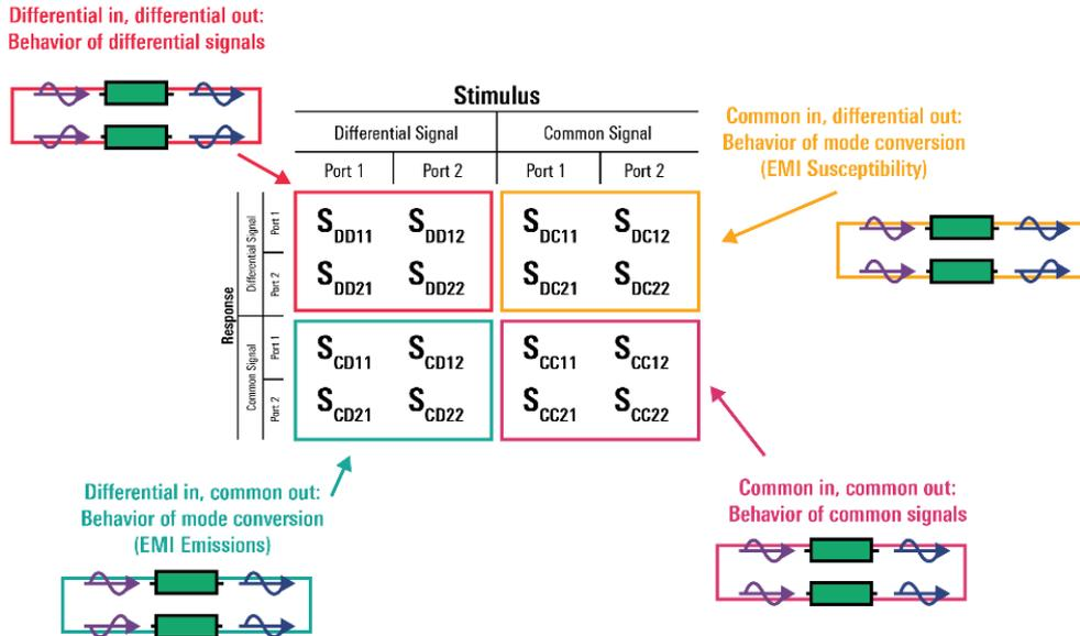
Figure 6: Differential S-parameters.
