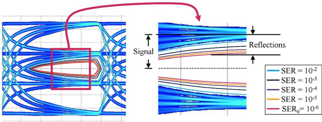
Figure 16: Like COM, also ERL is an SNR-like figure of merit, calculated from the measured S-parameters based on a defined model of the overall transmission system.
