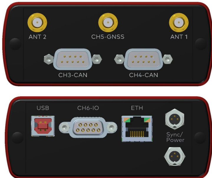
Figure 8 : VN4610 connectors layout
