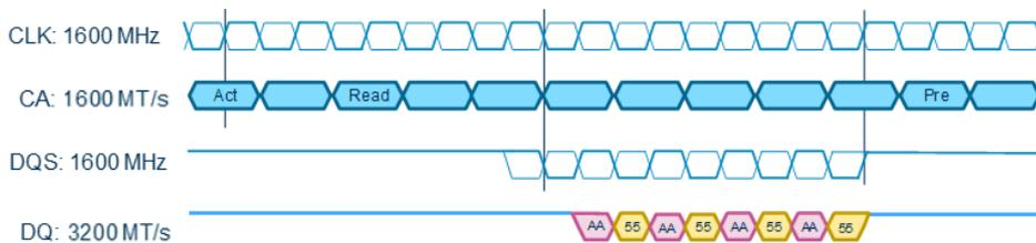
Fig. 2-9: Single data rate (CA) and double data rate (data) for DDR4 3200 MT/s (Read Burst)
