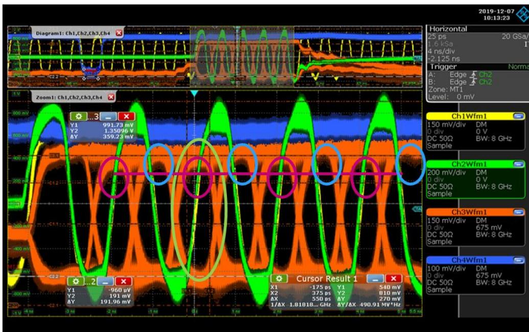
Fig. 3-11: Advanced triggering: two stage trigger with event count and Zone Trigger to capture DQ bursts with bit by bit overlay: odd bits have less margin (magenta Circles) than even bits (blue circle)
