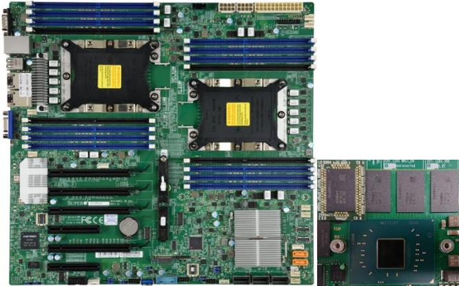
Fig. 2-3: Server system (left, scaled down) AND embedded device (right, scaled up)
