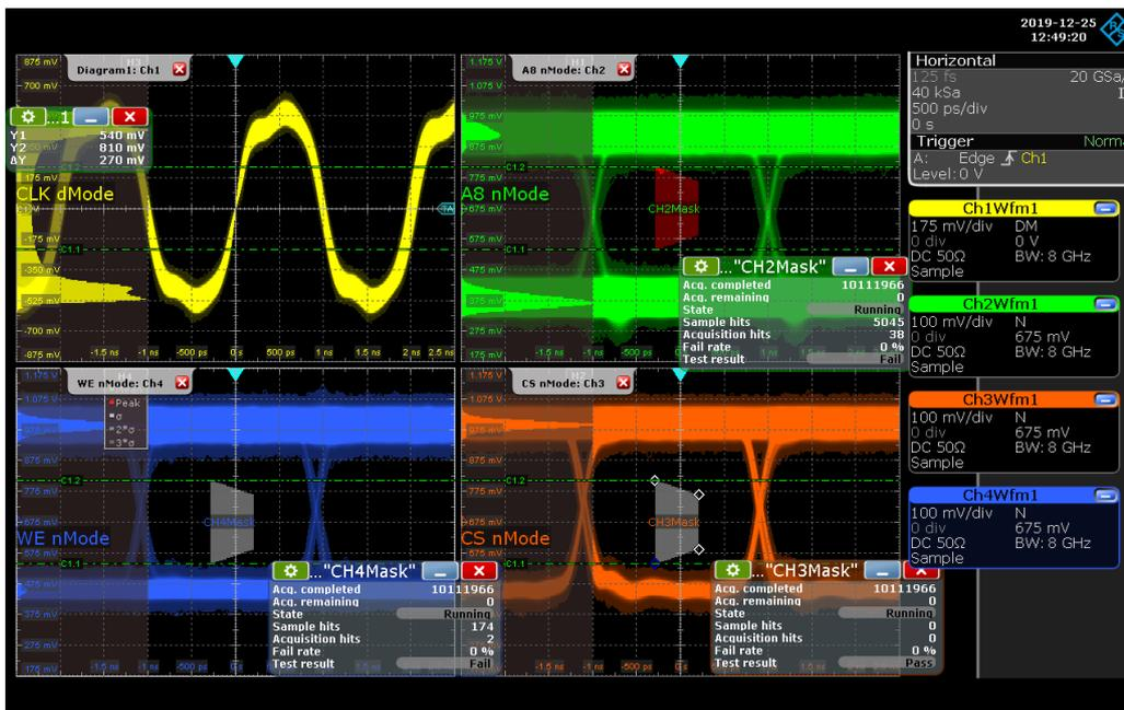
Fig. 3-12: Multiple eye diagrams and included mask tests with the fast acquisition of the R&S® RTP oscilloscope (edge trigger on CLK)
