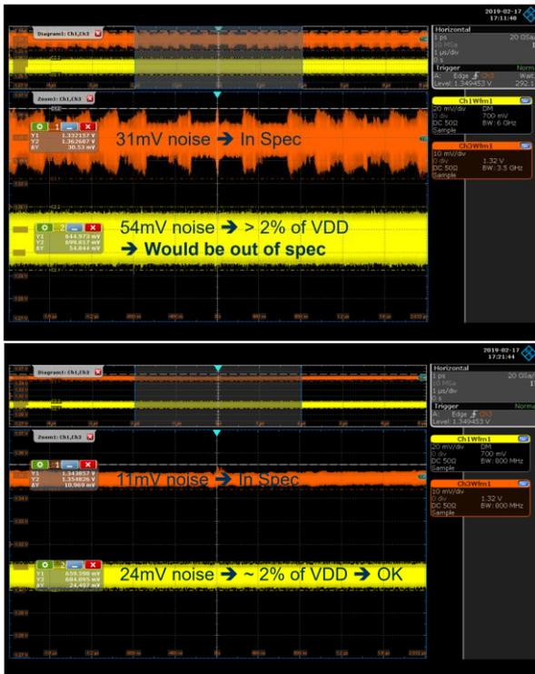
Fig. 3-19: VDD (orange) and Vref (yellow) noise at 6 GHz (above) and 800 MHz (below)
