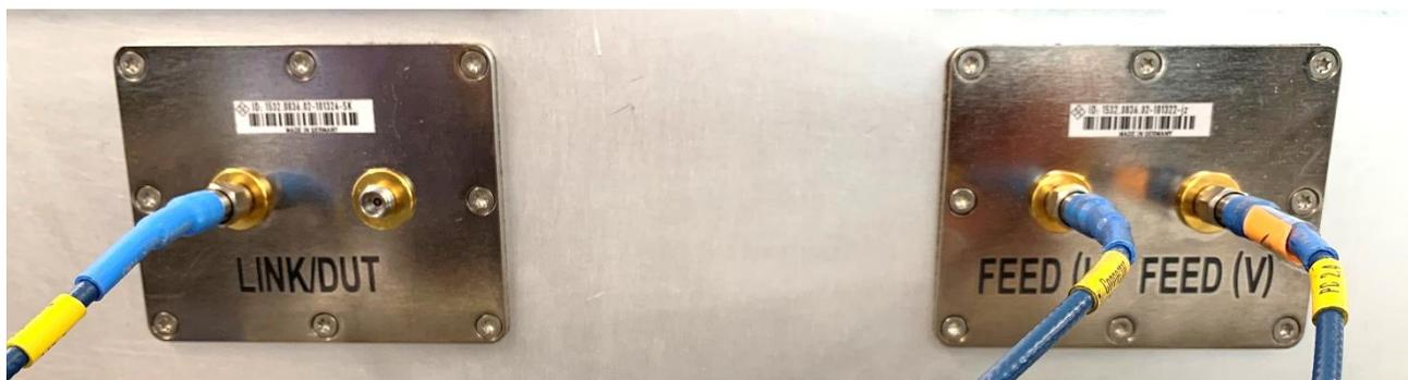
Figure 14: Feedthroughs R&S@ATS1800C
