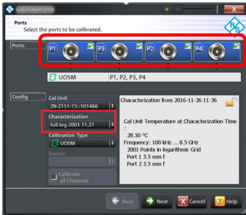
Fig. 3-3: Configuration for calibrating all four ports of the ZNB4
