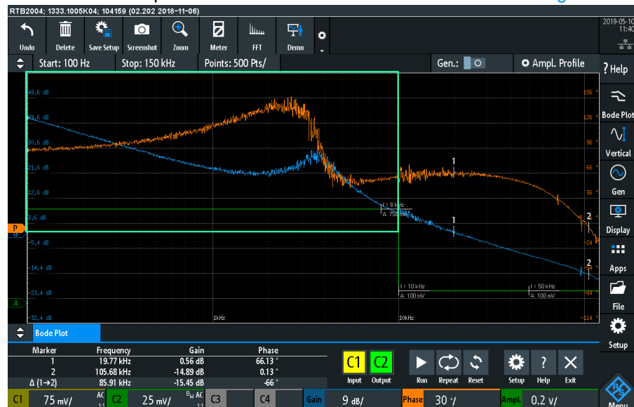
Fig. 4-2: Improved amplitude at lower frequency (Version 1)
