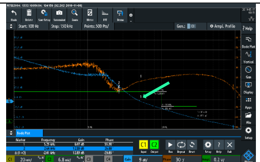
Fig. 6-9: CLR with additional output filter capacitance of 100 \mu F
