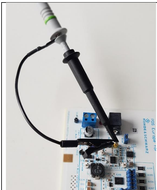
Fig. 5-3: Standard ground connection
