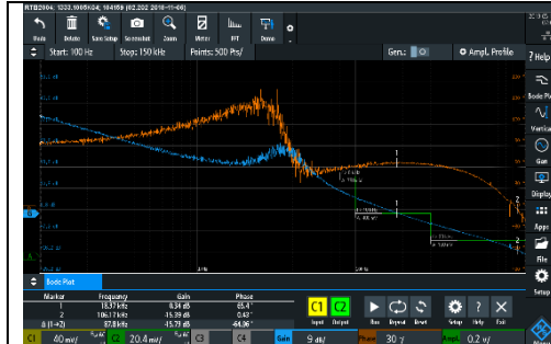
Fig. 6-3: CLR measurement @ Pout = 2,5W
