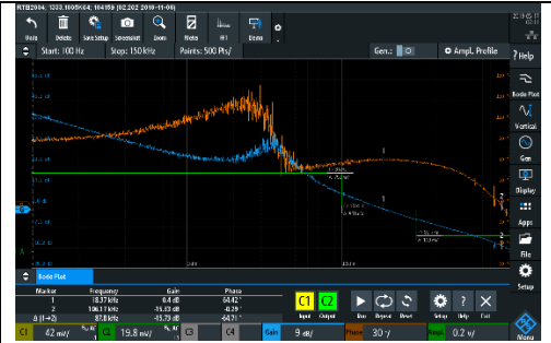
Fig. 6-4: CLR measurement @ Pout = 2W
