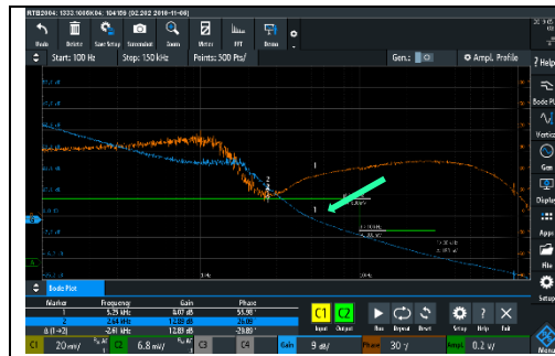
Fig. 7-5: Measured CLR with additional output filter capacitance of 100µF
