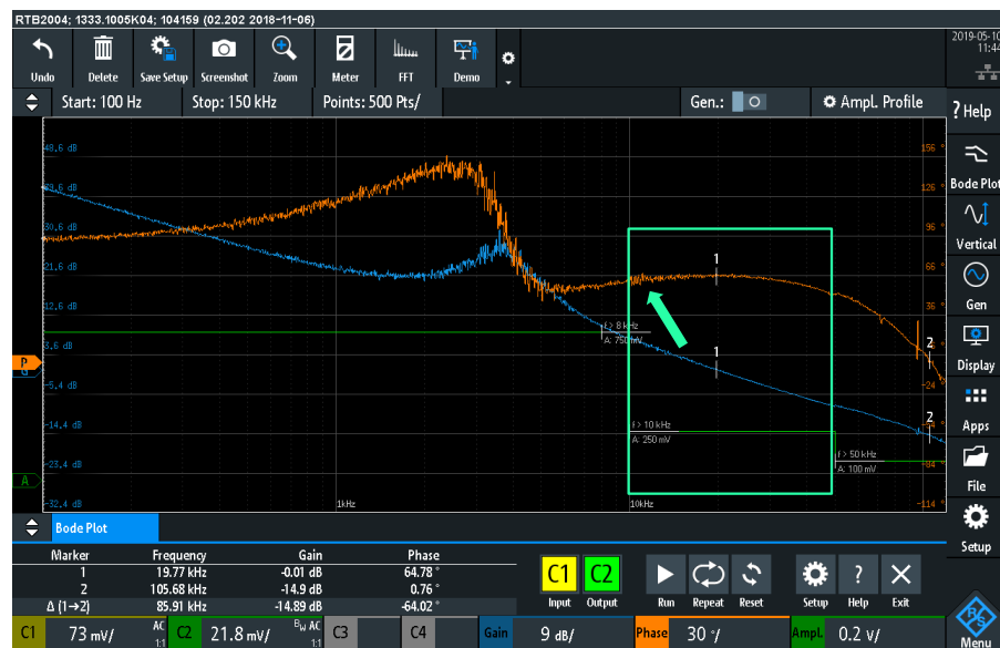
Fig. 4-3: Improved profile (Version 2)
