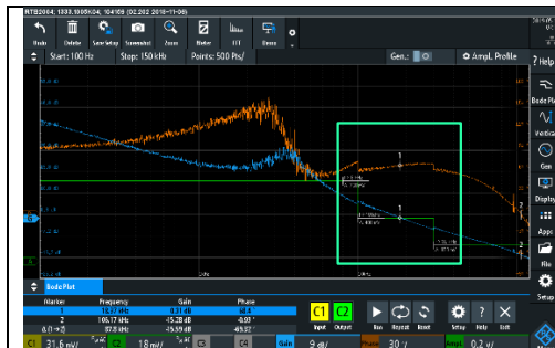
Fig. 6-5: CLR measurement @ Pout = 1,5W
