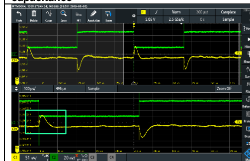
Fig. 7-3: Load transient test with standard output filter capacitance
