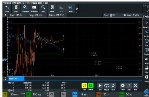
Fig. 6-7: CLR measurement @ Pout = 1W
