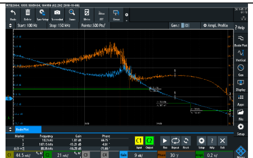
Fig. 6-6: CLR measurement @ Pout = 1,5W Improved Profile
