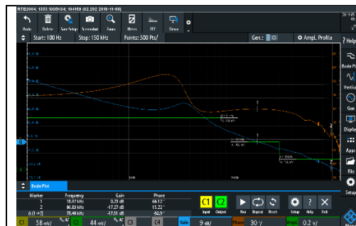
Fig. 6-1: CLR measurement @ V_{in} = 8V , P_{out} = 2,5W
