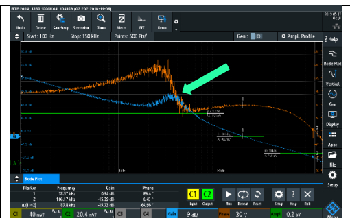
Fig. 6-2: CLR measurement @ V_{in} = 16V , P_{out} = 2,5W
