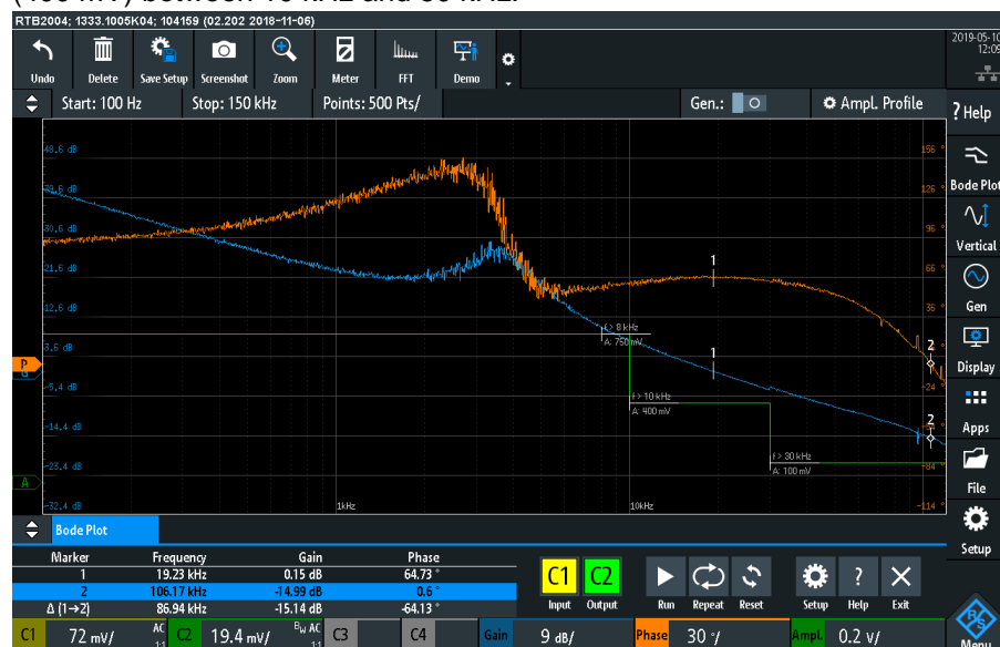
Fig. 4-4: Optimized amplitude profile
