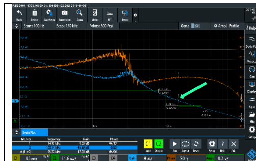
Fig. 6-8: CLR reference with standard output filter capacitance
