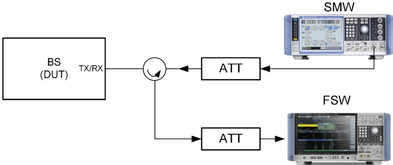
Figure 27: Test setup transmitter intermodulation
