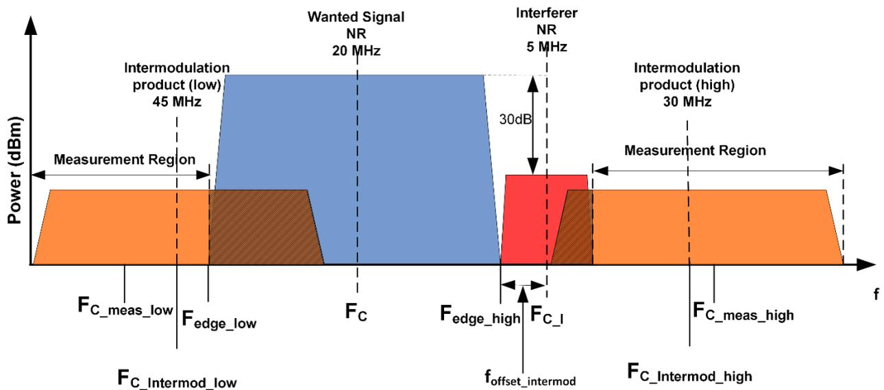
Figure 28: Measurement regions for the intermodulation test. Regions that overlap with the wanted signal or the interferer must be excluded
