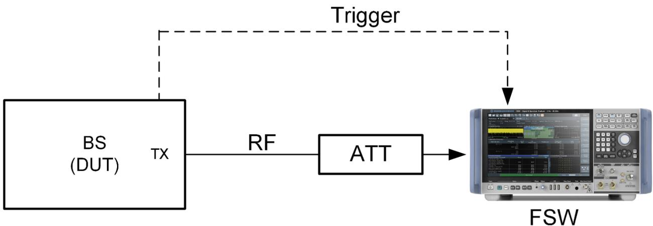
Figure 20: Test setup ACLR
