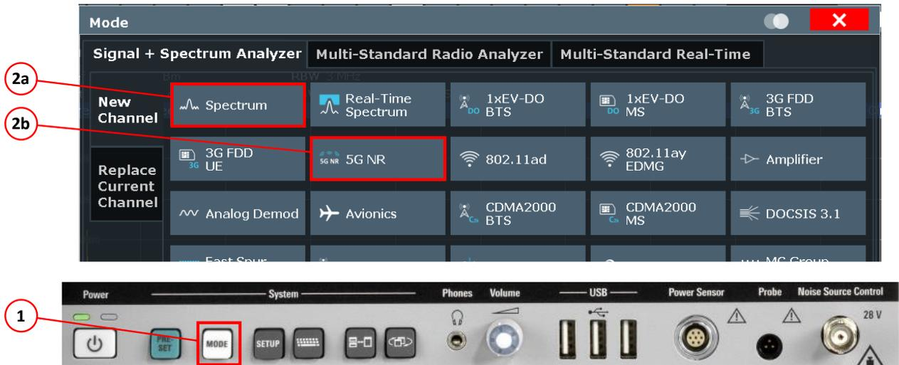
Depending on the operation mode, different measurements are available. What measurement is required for which test is specified in the respective section. Select the measurement by pressing **Select measurement** at the overview-screen or by pressing **MEAS** key on the front panel of the instrument.
