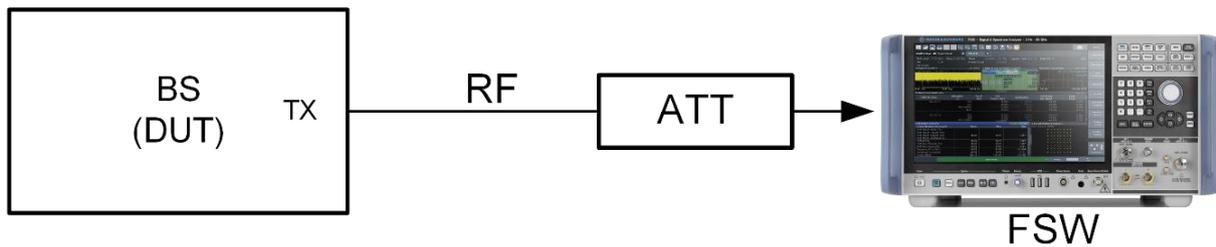
Figure 24: Test setup spurious emissions
