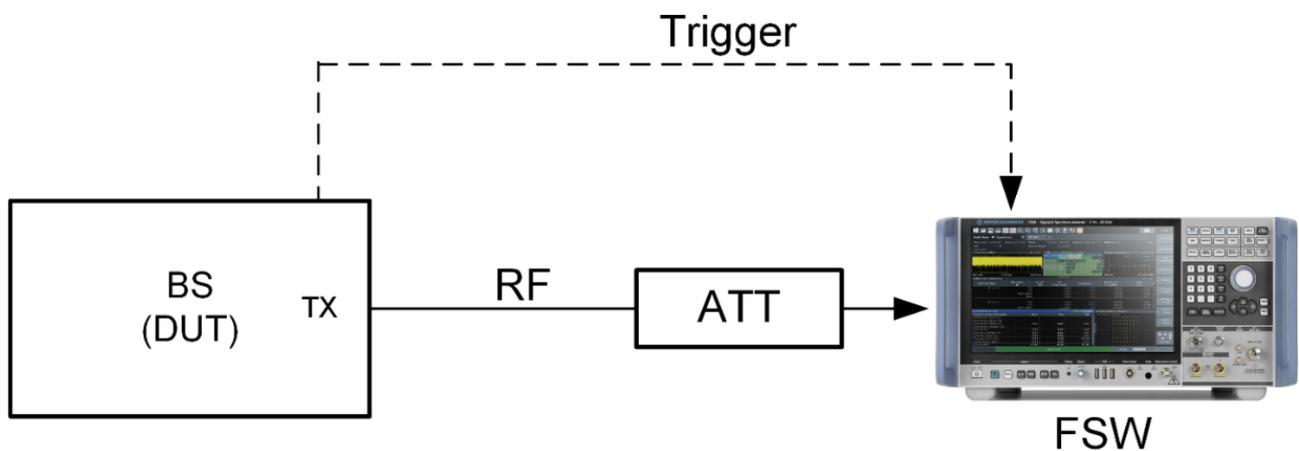
Figure 22: Test setup for SEM
