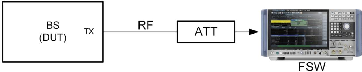
Figure 8: Test setup for total power dynamic range
