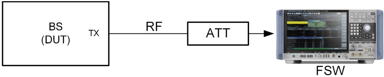
Figure 6: Test setup base station output power
