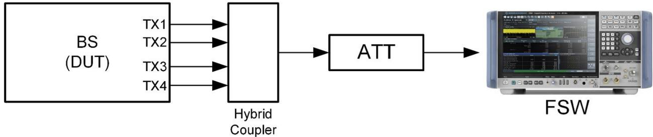
Figure 15: Test setup time alignment error
