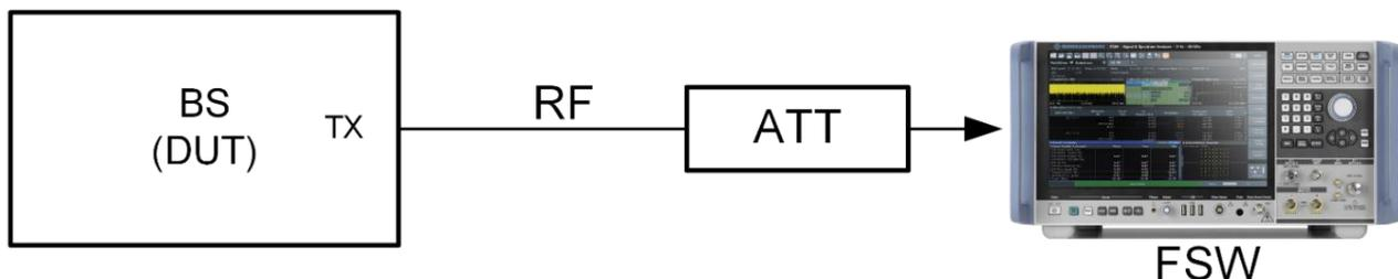
Figure 13: Test setup for frequency error and EVM
