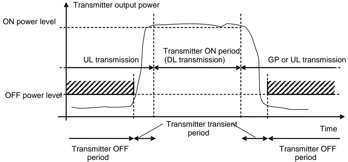
Figure 10: Definition of transmitter ON and OFF periods [1]
