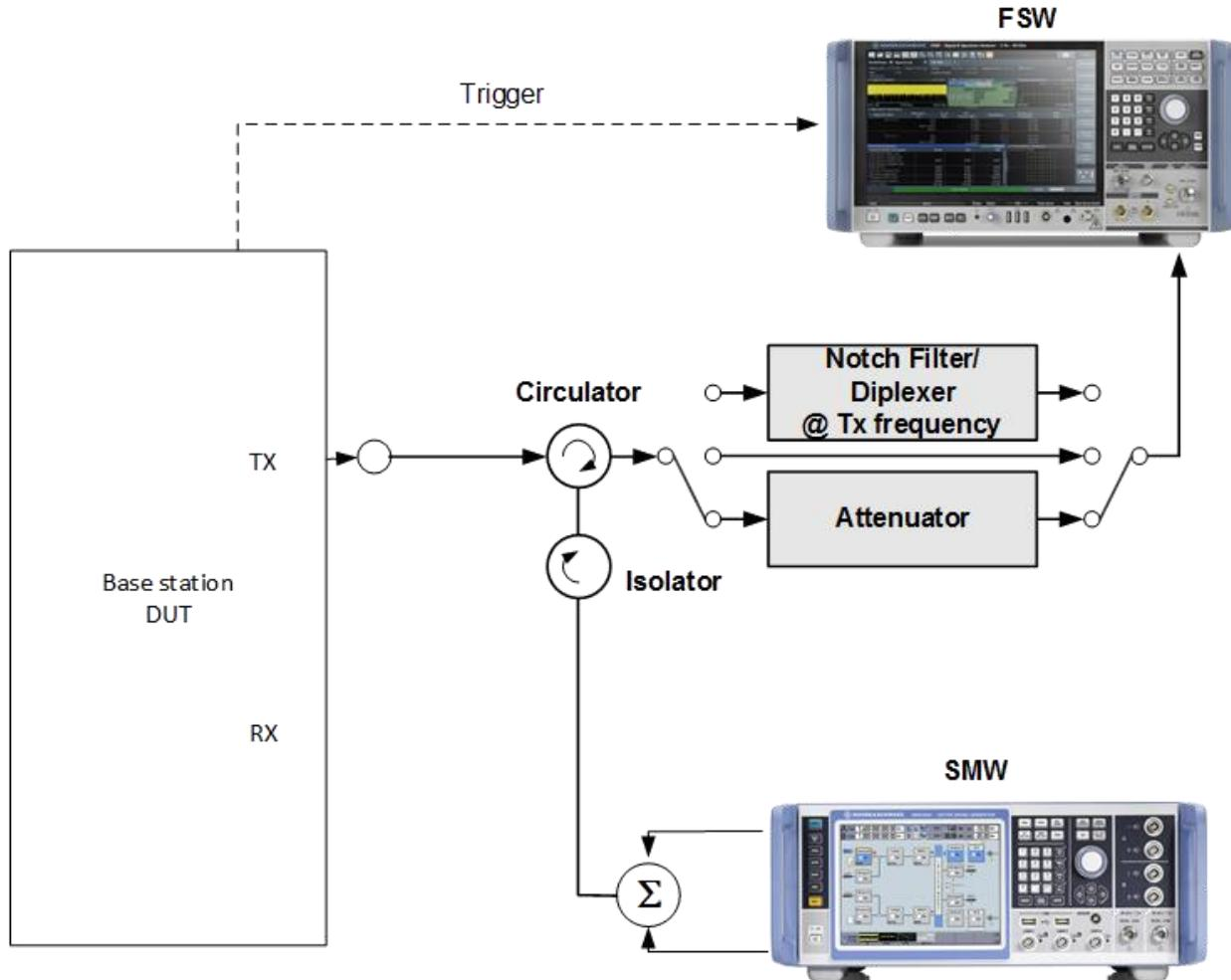
Figure 4: Complete Tx test setup overview
