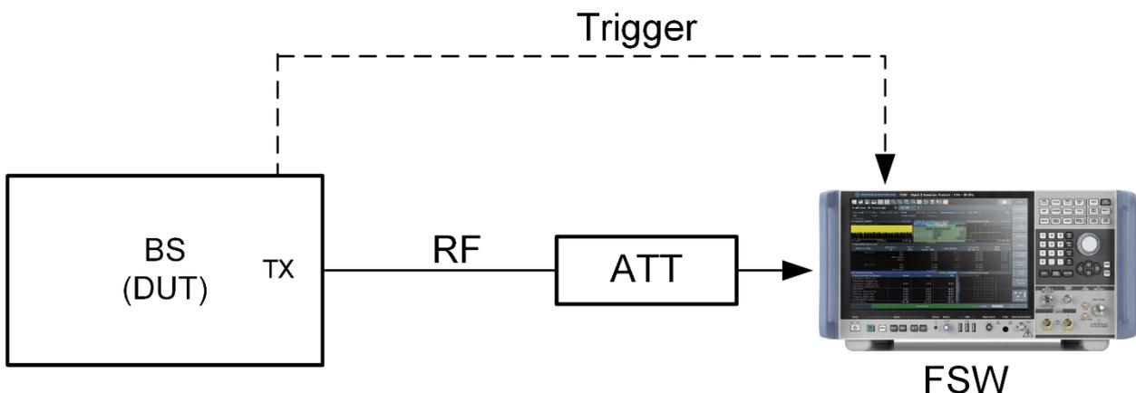
Figure 17: Test setup unwanted emissions
