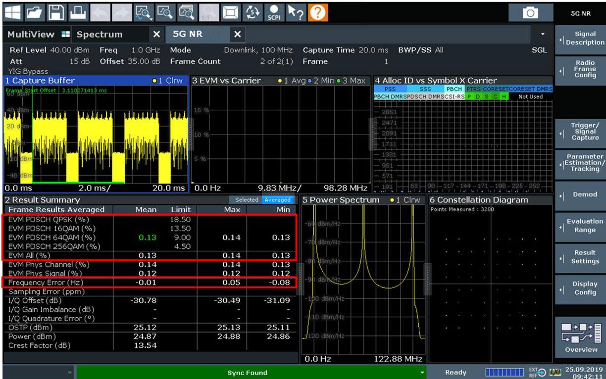
Figure 14: Frequency error (6.5.2) and modulation quality (6.5.3)
