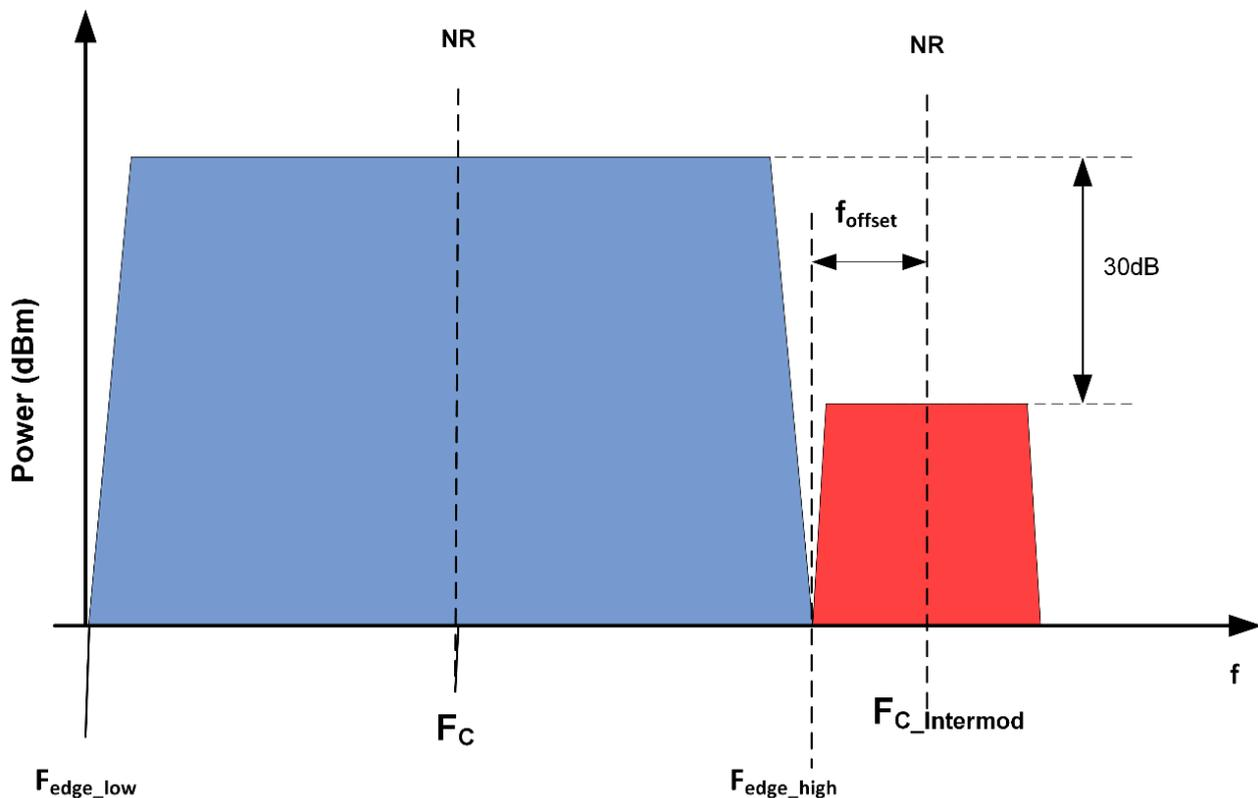
Figure 26: Transmit intermodulation
