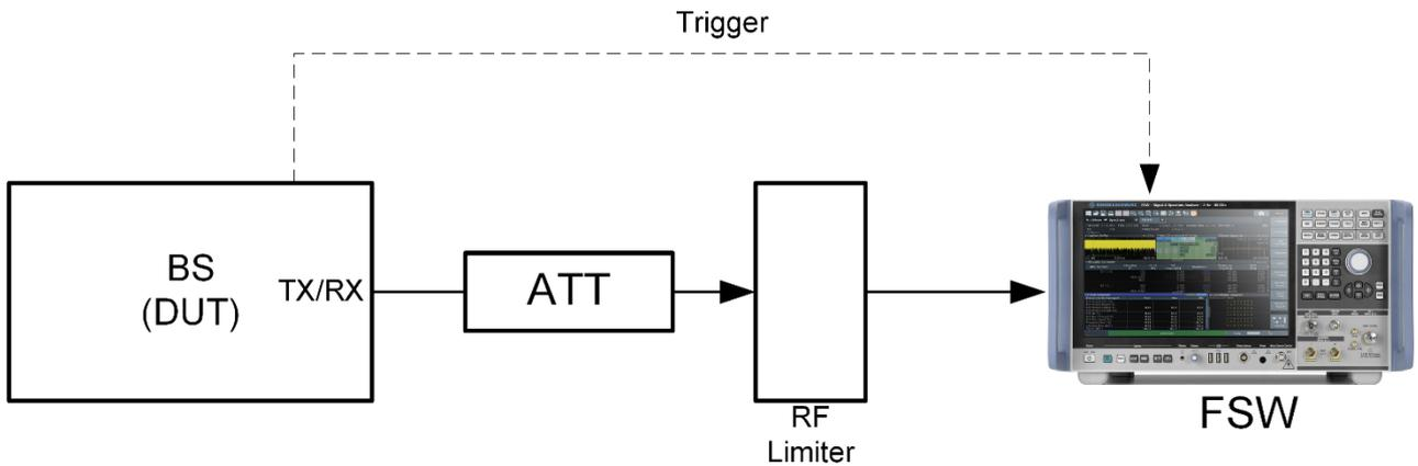
Figure 11: Test setup for transmit ON/OFF power measurements
