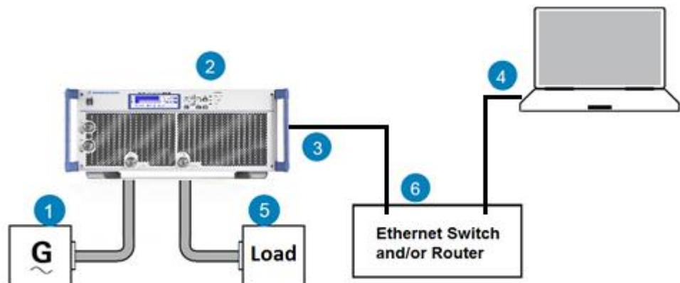
**Figure 2: Network configuration with a LAN switch and/or Router**
