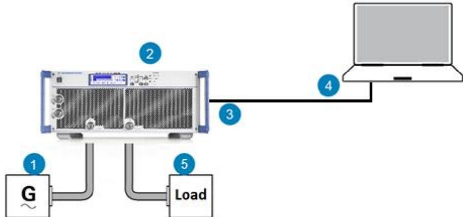
**Figure 1: Simple network configuration including Signal Generator and Load**
