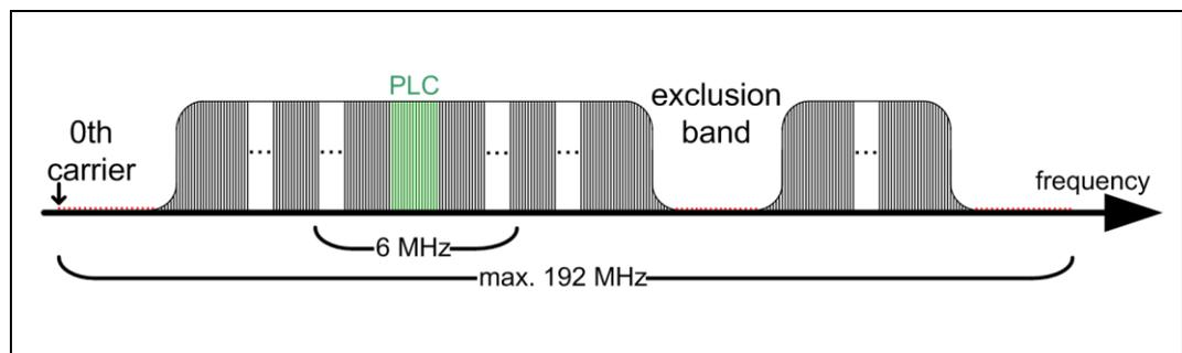
Fig. 8: Downstream signal with the 0th carrier, PLC and exclusion band.
