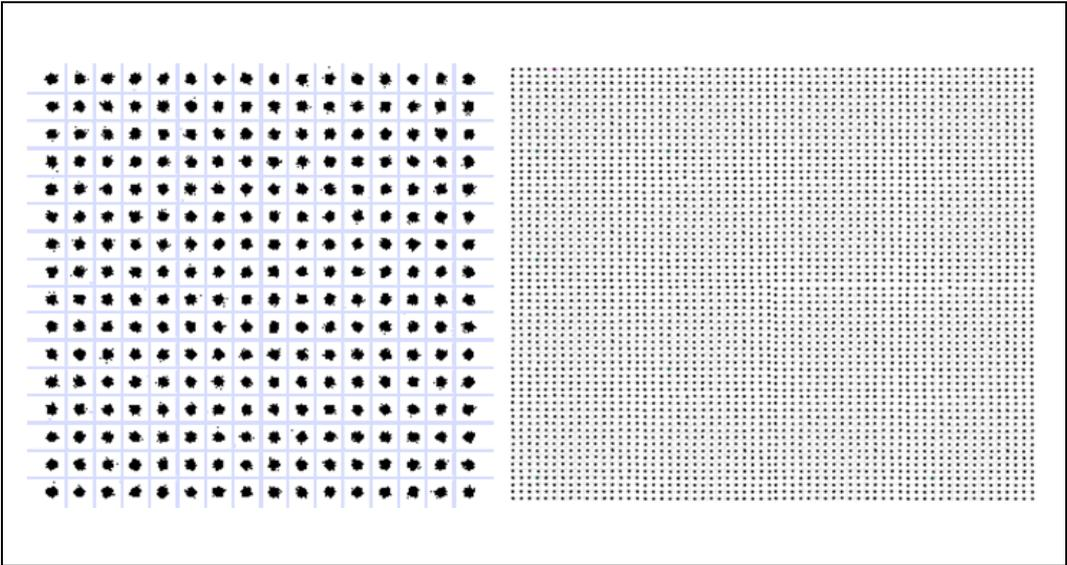
Fig. 10: Modulation order 256QAM (left) and 4096QAM (right).
