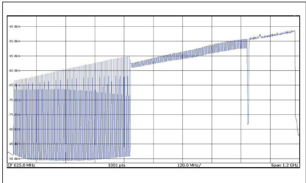
**Fig. 12:** Test signal for a cable TV amplifier with analog TV, QAM and a 192 MHz DOCSIS 3.1 signal with a total of 15 dB up tilt. The DOCSIS 3.1 signal contains the bulk of the power.
