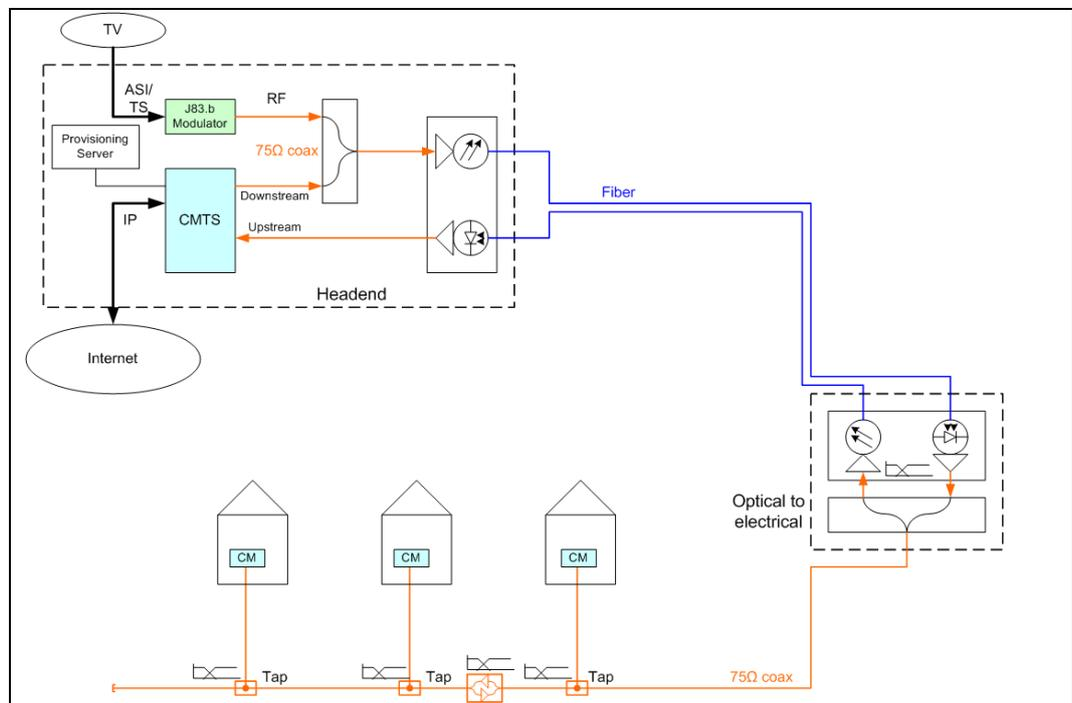
Fig. 1: Schematic diagram of the cable TV network.
