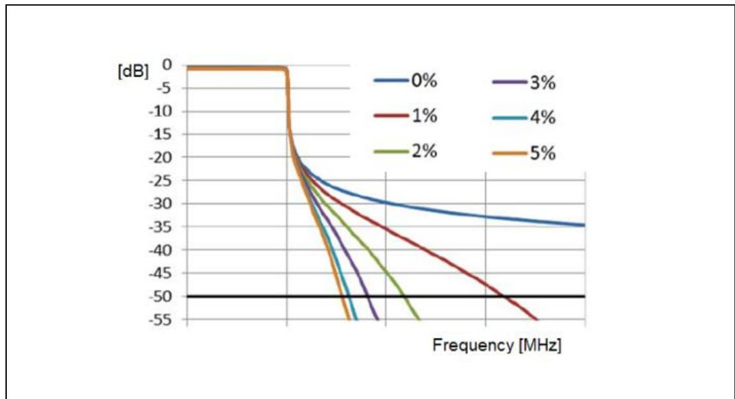
Fig. 6: Tukey raised cosine windowing with differing values.
