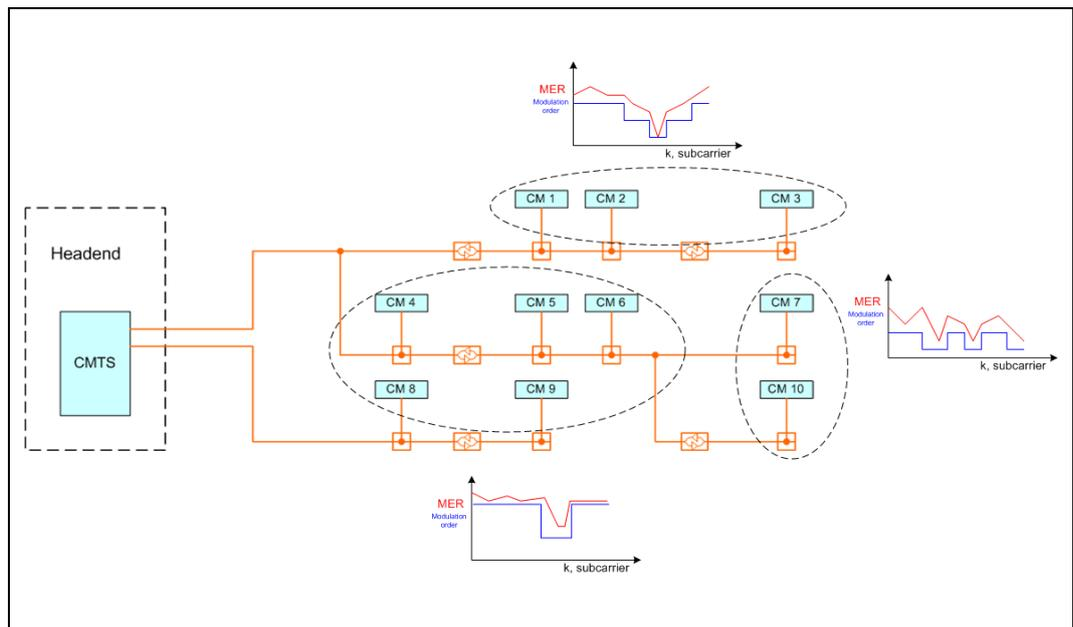
Fig. 9: Simplified schematic of an HFC network with varied MER values.
