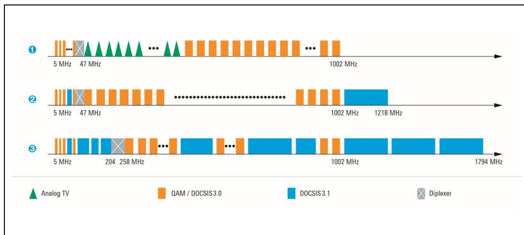
Fig. 2: ① Current channel assignment, ② channel assignment with initial phase of DOCSIS 3.1, ③ channel assignment with final phase of DOCSIS 3.1.
