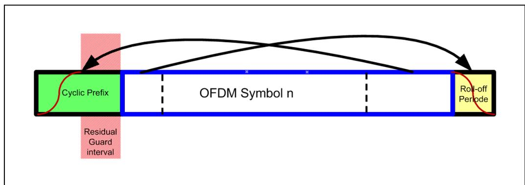
Fig. 7: Cyclic prefix and roll-off period of an OFDM symbol.
