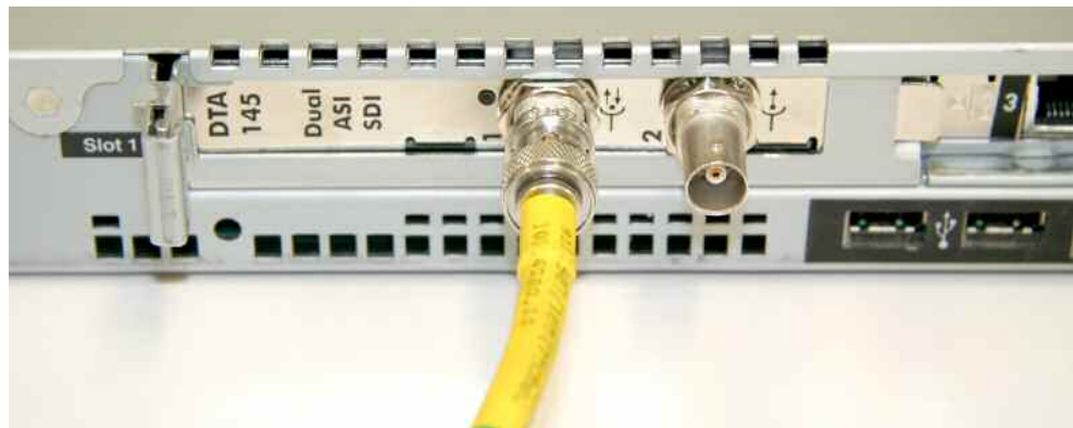
Figure 9: ASI input connection of the ATSC-M/H multiplexer
