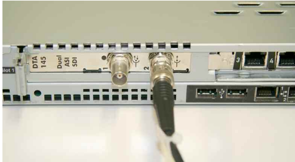
Figure 8: ASI output connection of the ATSC-M/H multiplexer
